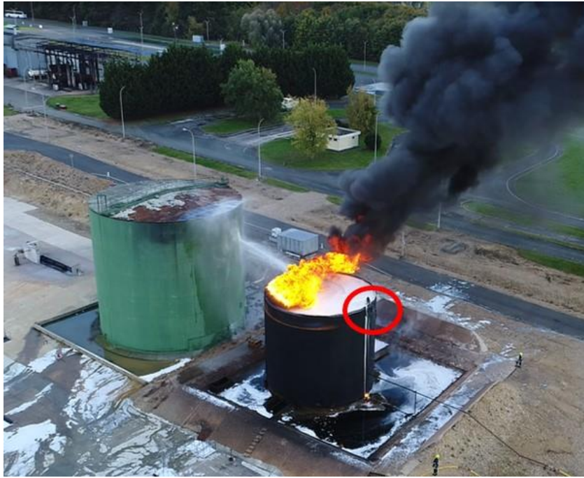
System application. (Pourer circled in red) Note control from "near side".
