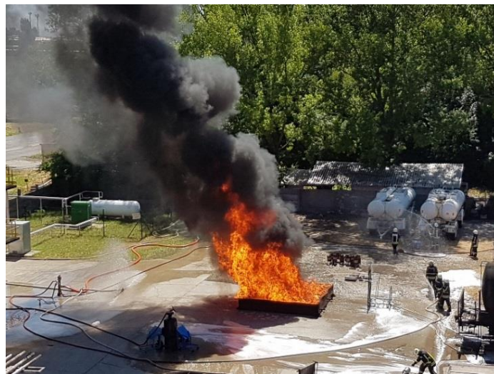
The “large” bund fire test
