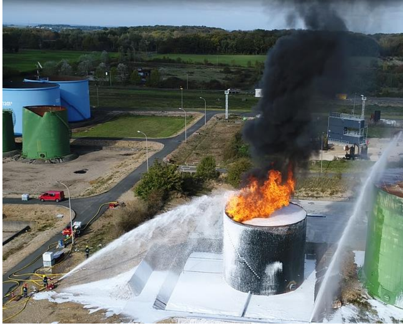
Monitor application to tank fire – note build-up of foam from “rear” wall
