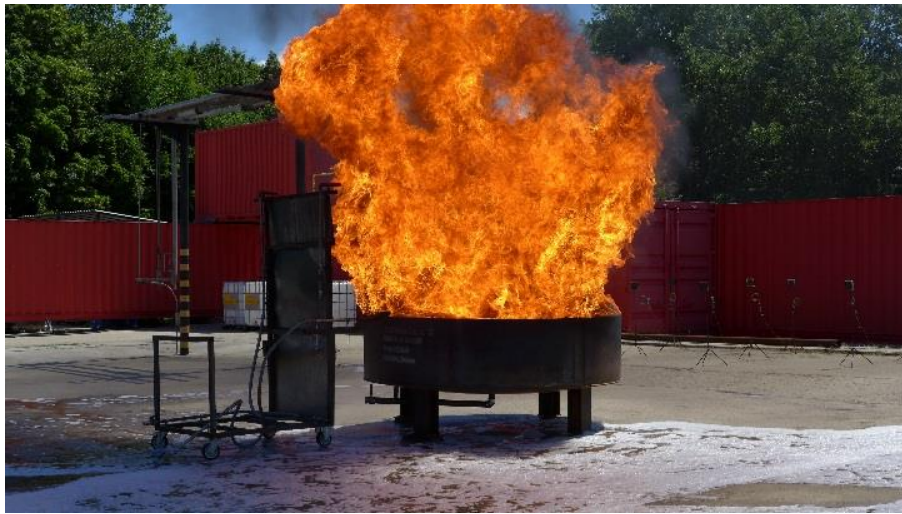
The standard LASTFIRE test pan
