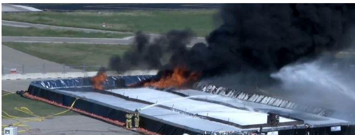
40m test CAF pouter application “virtual extinguishment”. Note back up pouter not yet actuated and remaining fire outside the actual test pan (due to fuel leaking into secondary containment from a fuel line.)
