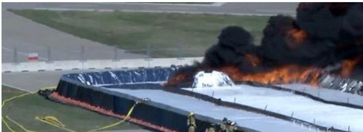
Back up pourer operating after extinguishment
