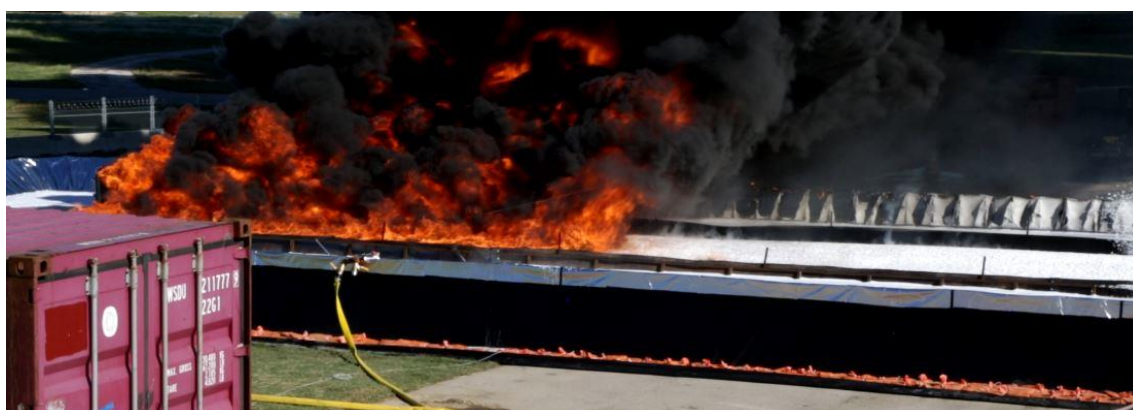
40m test CAF pouter application – extinguishment to ~30m
