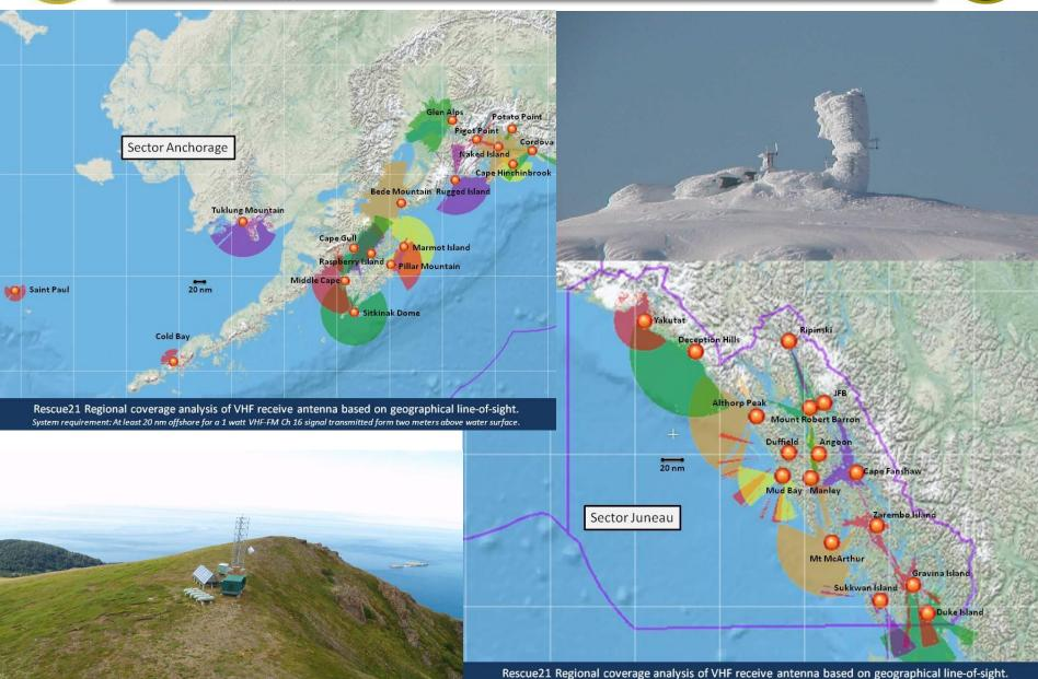
System requirement: At least 20 nm offshore for a 1 watt VHF-FM Ch 16 signal transmitted form two meters above water surface.
