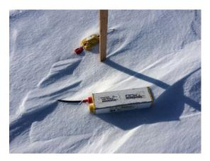
**Receiver Operation** Receiver crew lays out and pick up a grid of receivers on the tundra. 660ft x220ft grid
