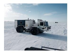
**Source Operation** Seismic vibrator trucks working a dense grid on the tundra 110 ft x110ft grid
