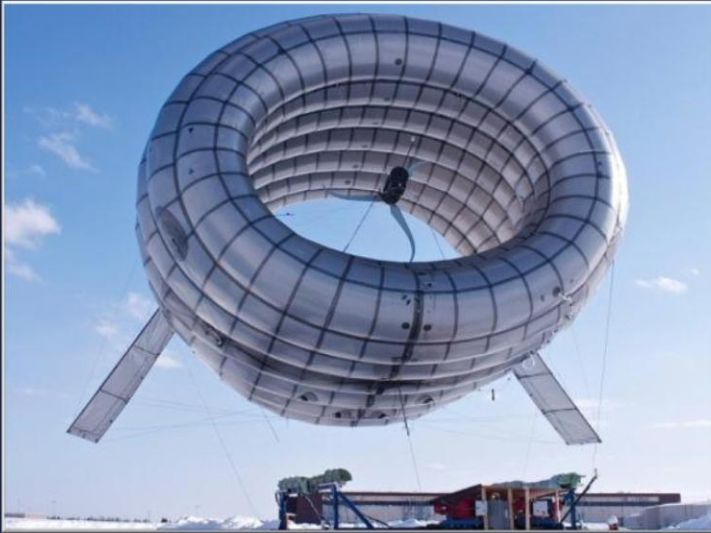
Altaeros Energies Helium Balloon Wind Turbine
