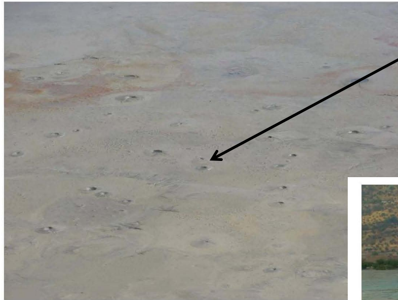
Figure 11.11. March 9, 2010 Sand Boils in Tailings about 10 m Upstream of Ovejeri (S33.052016°, W70.798687°)
