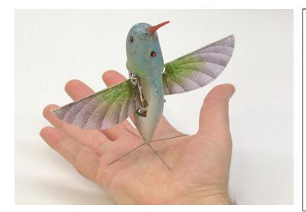
AeroVironment's advanced unmanned aircraft systems are used by the US Department of Defense and allied military services to provide real-time, airborne reconnaissance, surveillance and communication. Its 6.5 inch tall nano-hummingbird prototype aircraft is the first to operate using only its flapping wings for propulsion and control. The 2/3 ounce aircraft is capable of flying in all directions and can fit into tight spaces.
