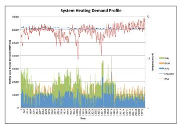
**Figure 20.** System Heating Demand Profile (Temperature is plotted on a logarithmic axis to highlight low temperature trends.)
