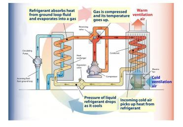
Figure 1. How a Heat Pump Works<sup>iv</sup>
