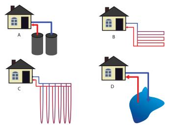
**Figure 2.** Ground-loop configurations: a) open-loop borehole, b)closed-loop horizontal, c) closed-loop vertical, d) open-loop pond water back to the original well or elsewhere.
