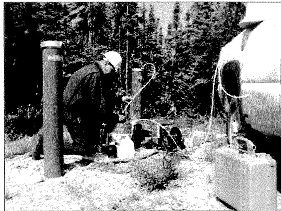
A field technician performs groundwater sampling from a monitoring well at Flint Hills Resources' North Pole refinery in 2013. Results from this sampling will be included in the site characterization report that FHRA will submit to DEC in December 2013. (FHRA photo)
