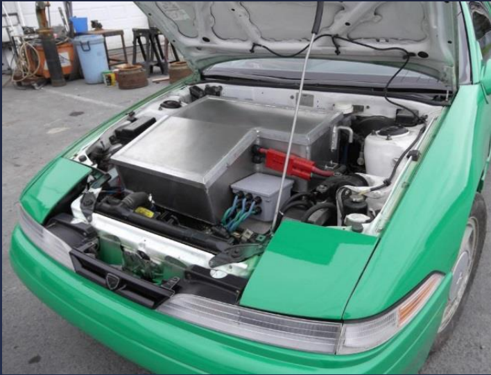
Modified '97 Eagle Talon EV Test bed
