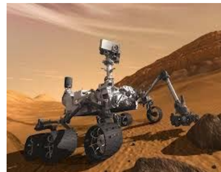
The Mars vehicle Curiosity carries a radioisotope power system that generates electricity from the heat of plutonium's radioactive decay. Because it does not rely upon solar cells it can roam the Red Planet for at least 697 days.
