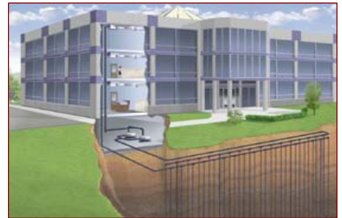
Schematic rendering of closed loop geothermal heat pump system. Image from www.mcquay.com
