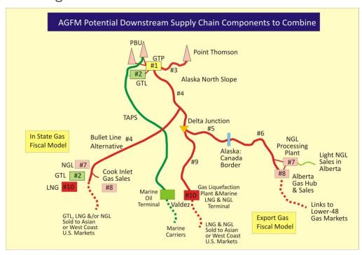
Components "1", "2", "4", "7", "8" and "10" can be reconfigured to model gas export routes or to model In-State "Bullet Line" gas supply to Cook Inlet with optional NGL, GTL and / or LNG plants placed there for exports.
