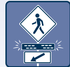
Rectangular Rapid Flashing Beacons (RRFB)
