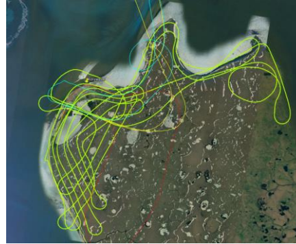
Flight lines and view from plan, Matt Nolan collecting aerial photos to support orthoimagery and topography collection for State of Alaska
