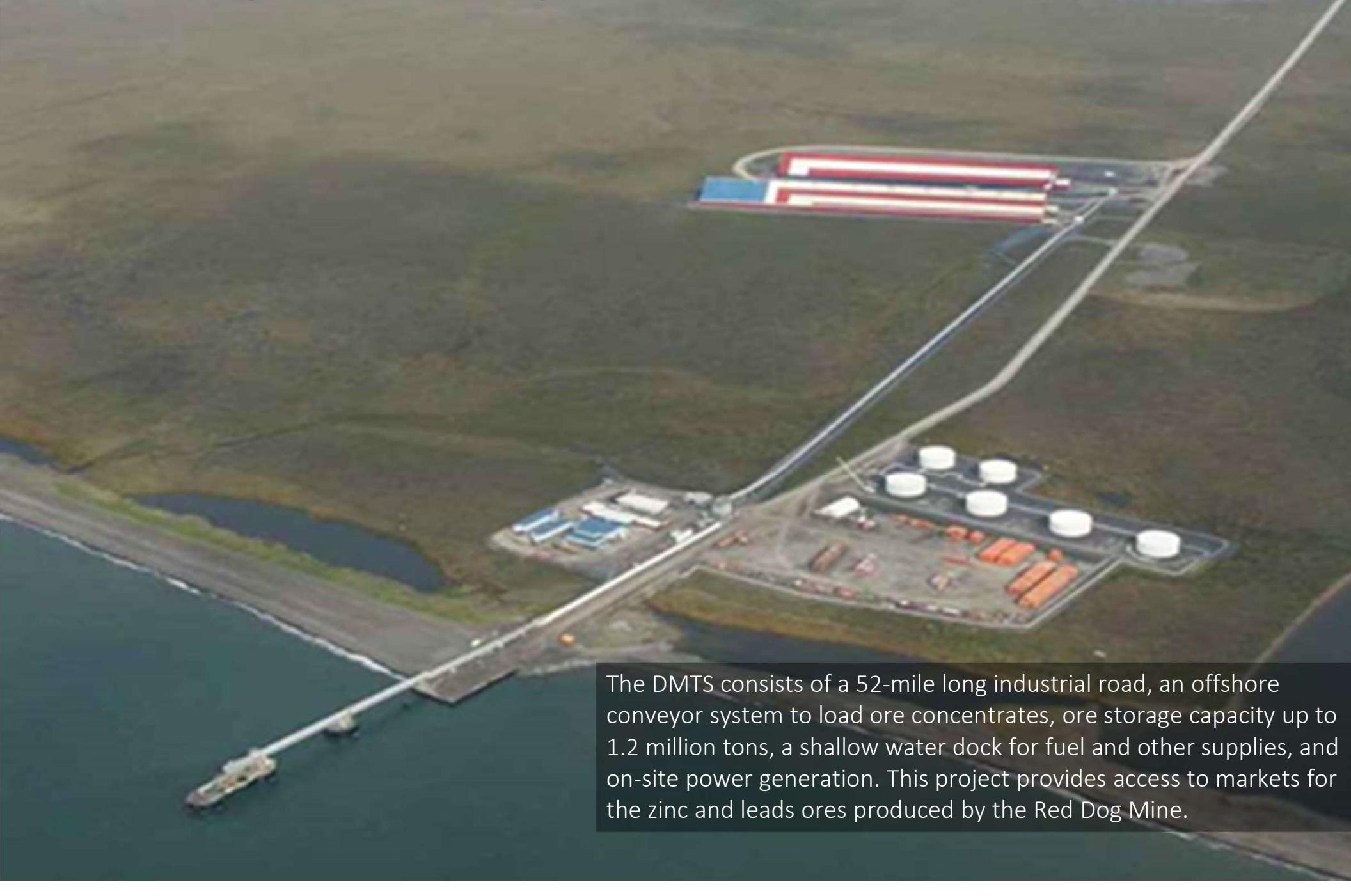
The DMTS consists of a 52-mile long industrial road, an offshore conveyor system to load ore concentrates, ore storage capacity up to 1.2 million tons, a shallow water dock for fuel and other supplies, and on-site power generation. This project provides access to markets for the zinc and lead ores produced by the Red Dog Mine.
