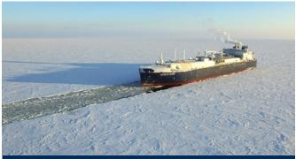
The first generation design of Arctic LNG carriers is extremely capable in ice and can sail independently through 2.1-metre-thick ice. The fifteen carriers, built to date, can manage on the NSR from July to December, whereas the second generation will manage year-round with a high transit speed through ice. In January 2021, three of the existing vessels undertook a test voyage along the NSR without icebreaker escort.
