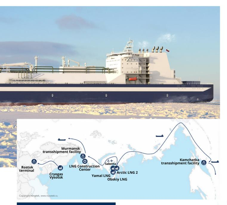
Transportation from Yamal LNG will, in the future, focus on the west-bound route to Europe, and from Arctic LNG 2 on the east-bound route to Asia along the NSR. The new Arc7 design allows transportation all year round on this challenging itinerary.
