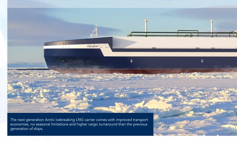
Construction of the next generation icebreaking LNG carriers will begin in South Korea later this year. From 2023, all six Arc7 classed vessels will be ready to transport liquefied natural gas from the Gydan Peninsula year-round along the Northern Sea Route, improving overall cost-efficiency of the transportation system.
