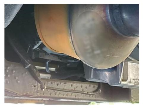
Both Police Departments provided city mechanics to etch and paint catalytic converters based on where the vehicle is registered. The mechanics worked together to take a photo of the vehicle's VIN and etch it onto the converter. They would then use high-temperature paint to mark the converter that indicates the jurisdiction. The entire process took about five minutes per vehicle.
