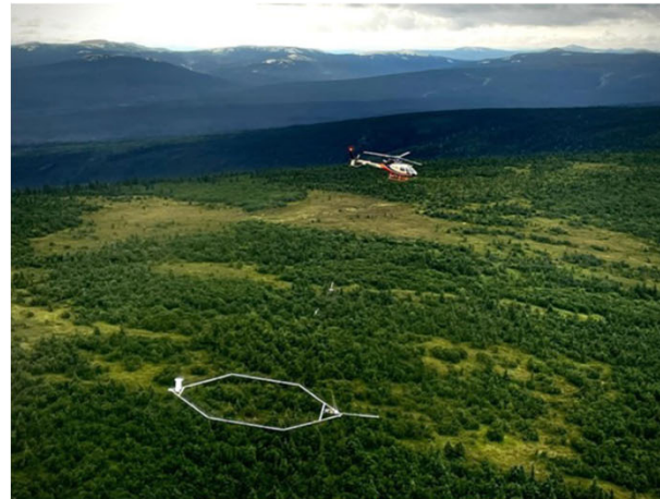
Photo: An airborne electromagnetic data acquisition (credit: Frederic Ladouceur, SkyTEM Canada Inc.)
