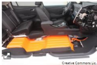
The lithium-ion battery in a Nissan Leaf.
