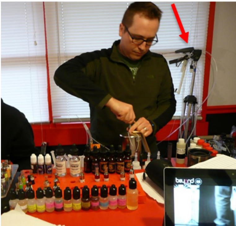
Figure 2. A National Institute for Occupational Safety and Health (NIOSH) investigator preparing to collect an air sample. An area sampling station is next to the window behind juice bar. Photo by NIOSH.
