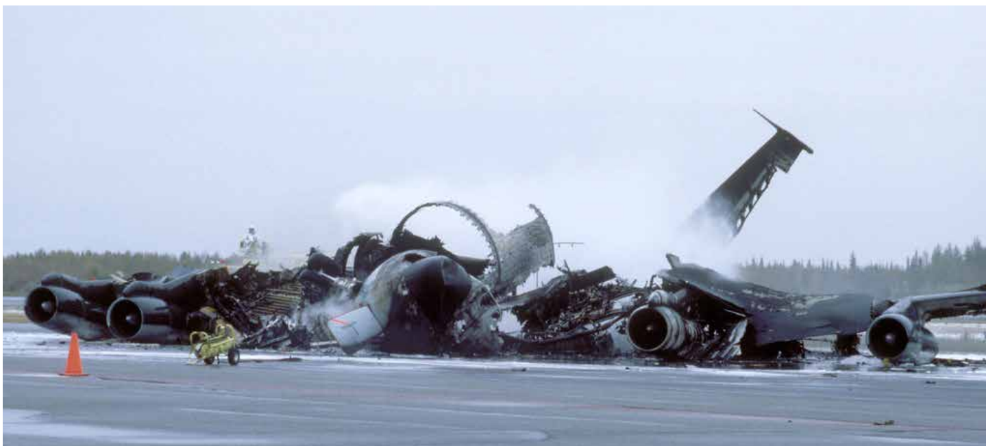
Crash crewmen spray a foam/water agent on the remnants of an Alaska Air National Guard KC-135E Stratotanker aircraft that exploded and burned on September 20, 1989 at Eielson Air Force Base while taxiing to a parking area. Photo: The U.S. National Archives
