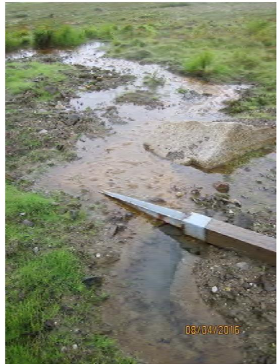
**Figure 4: Artesian flow at DDH 9475, drilled in 2009.**
