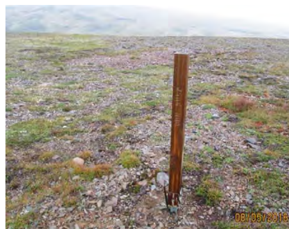
Figure 4. Monument marker. A wooden post with the drill hole number is commonly placed where the drill casing has been removed.
