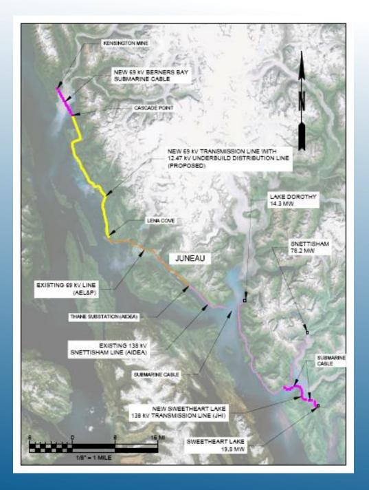
**Current Juneau Transmission** System only covers half of the CBJ. Lynn Canal **Transmission and** Juneau Hydropower line segments would roughly double the transmission grid of CBJ
