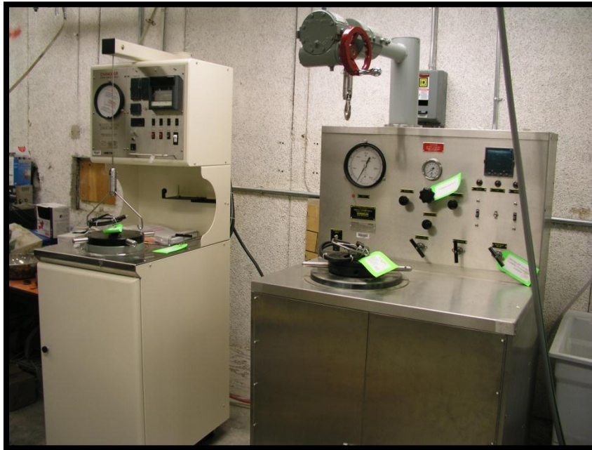
HPHT Consistometer and Curing Chamber used simulate well temperatures and pressures.
