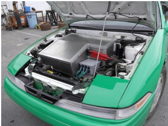
Converted '97 Eagle Talon EV testbed
