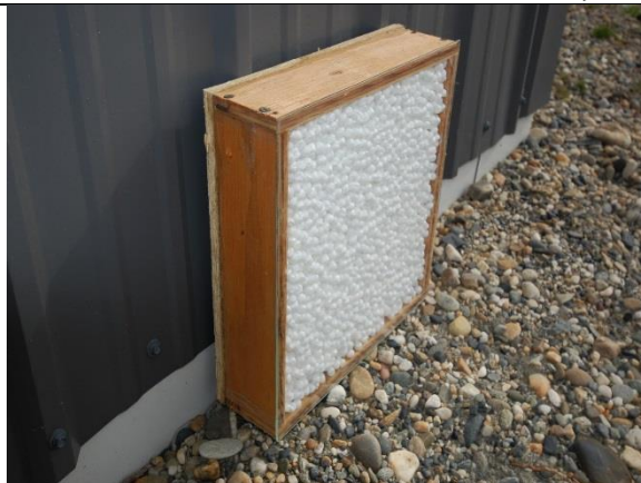
UV stability test of the EPS beads
