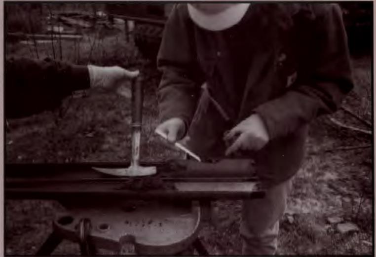
**A commercial drilling contractor may be employed to collect core samples during the site investigation phase of a cleanup. This soil core sample will be analyzed in a laboratory to determine its properties and detect specific contaminants.**
