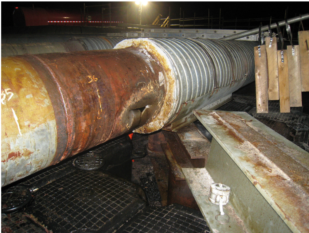
Photo showing the puncture in the BPXA DS 16 Flowline D and the wooden blocks to prevent the flowline from shifting. (Photo courtesy of BP)
