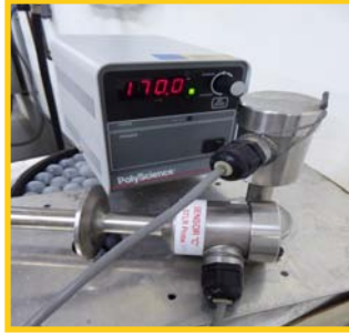
A recording thermometer is used to monitor milk temperature during pasteurization.
