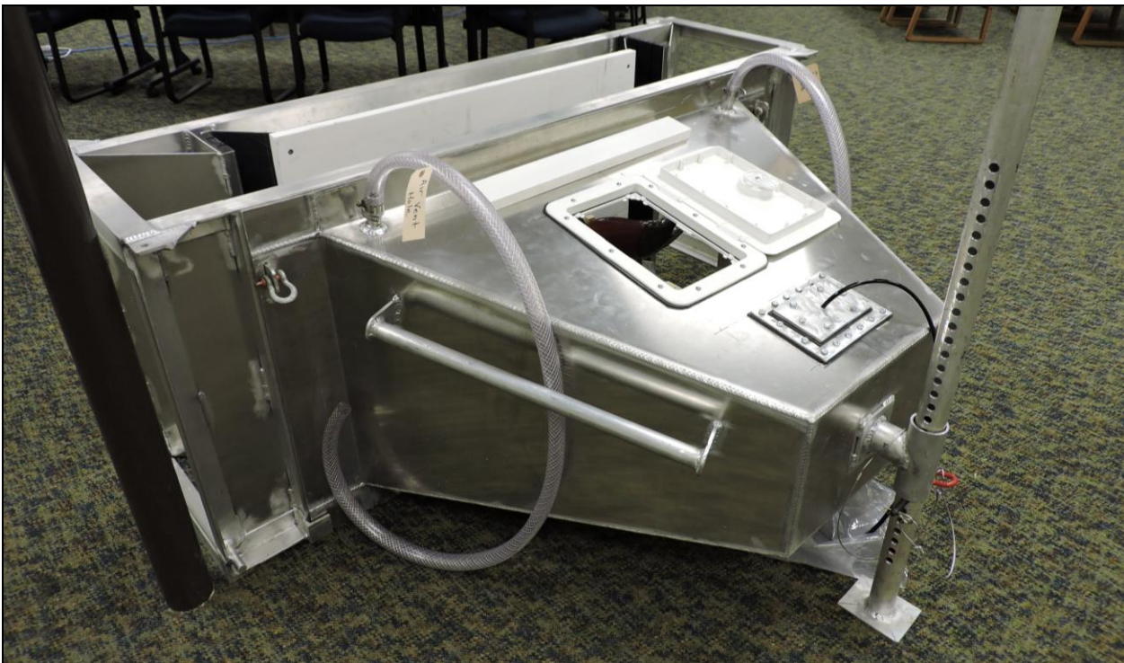
Figure 5: Video weir camera box and passage chute.
