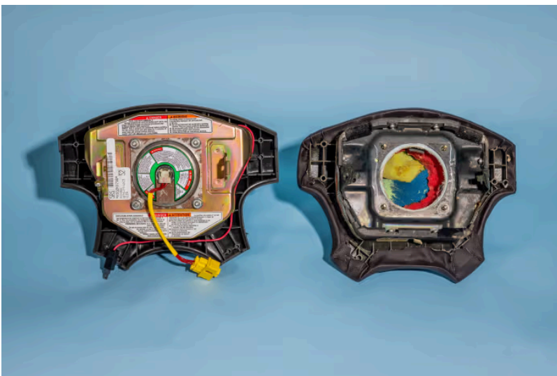
At American Honda Motor in Torrance, Calif., an example of a certified air-bag module next to a counterfeit air-bag module filled with colored foam. PHOTO: ROGER KISBY FOR THE WSJ
